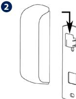
Place the sensor above the hook and slide it into position.
