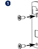
Position the wall bracket and secure it using the supplied screws.
