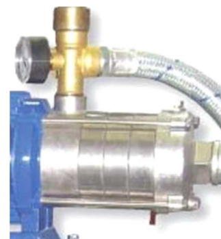
Fig 5: multistage pump outlet with manometer to replace with the transducer
