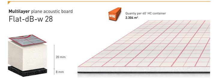
Insulation plate tacker panel Flat-db-w 28 made of expanded polystyrene EPS, declared thermal conductivity  $\lambda$  0,034 W/mK (EN 13163; EN 12667). The insulation panel is coated on the underside with a granulated SBR-rubber sheat to give exceptional acoustic performances. The upper side of the panel
