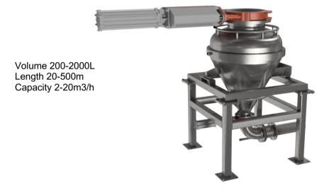
Blow Gun Cannon TOR is a pneumatic pipe conveying system made in Sweden since 1955. TOR uses compressed air for powerful handling of many kinds of materials for long and high distance. Dry, wet or heavy and abrasive materials are transported via conveyor pipes for compact installation. In line pipe switch diverters can direct the materials from several cannon senders to several cyclone receivers at different places. TOR can be used as vacuum conveying system.
