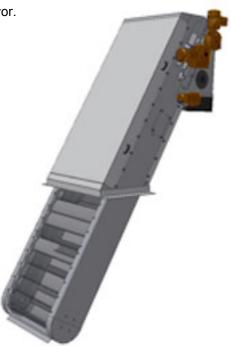
Through Flow Screen TFS separates solids (screenings, rubbish) from water. A band of linked perforated or mesh panels filters the water. Separated material is conveyed upwards and gets brushed/flushed off at the discharge point.
