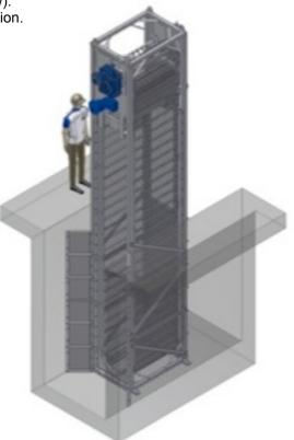
Center Flow Screen CFS separates solids (screenings, rubbish) from water. A band of linked perforated or mesh panels filters the water. Separated material is conveyed upwards and gets brushed/flushed off at the discharge point.
